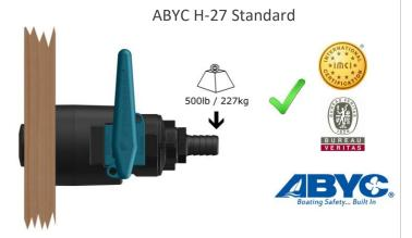
In accordance with ISO 9093-2 standards, Skin Fittings (Thru Hulls) are subjected to a 155kg (341.7lb) load, applied to the threaded section for a minimum of 30 seconds, without any damage occurring. TruDesign Skin Fittings (Thru Hulls) meet this standard.
